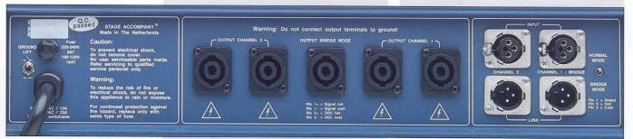
For those situations where really massive power into 8  $\Omega$  or 4  $\Omega$  is needed, the SA 1600 is equipped with a bridge mode toggle switch. Under music or speech conditions this increases power to 1600 W peak into 8  $\Omega$  and 2,200 W into 4  $\Omega$ . Some speakers on the market are able to withstand this power due to the aforementioned high crest factor of most music. With appropriate processors this will result in a headroom of about 10 dB.
